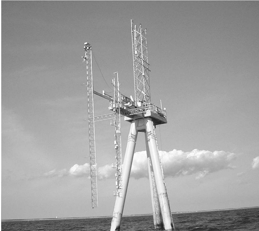
FIG. 1. The Air–Sea Interaction Tower with twin masts deployed during the CBLAST field campaign. Sonic anemometers mounted on the left (forward) mast translate vertically to obtain fine spatial resolution of the mean velocity and scalar profiles, while fixed sonic anemometers attached to the right (rearward) mast are used to measure vertical (turbulence) fluxes of momentum and scalars.
