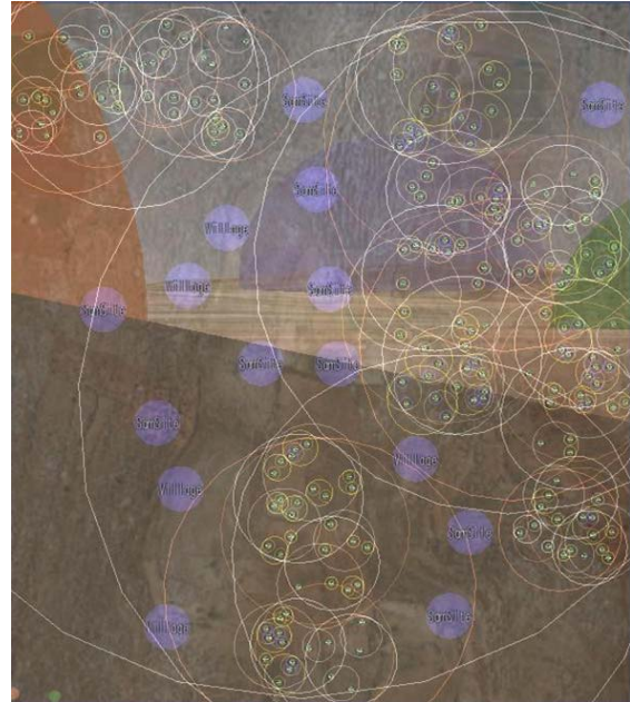
Figure 69. Proto partitions target set into hierarchical subproblems, indicated here by circles.
