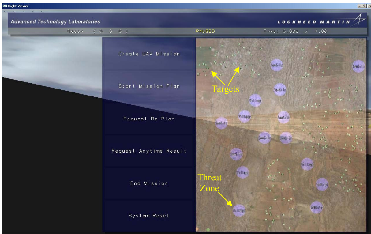
Figure 68. PCAA Mission Planning Application Flight Viewer, showing the terrain with targets and threats. Targets are green points, while threat zones are purple.
