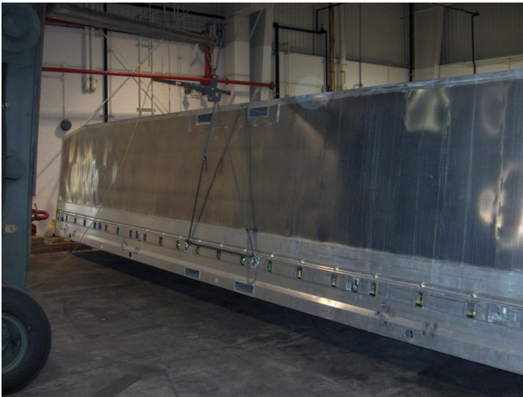
Figure 8. Rotational edge drop.
