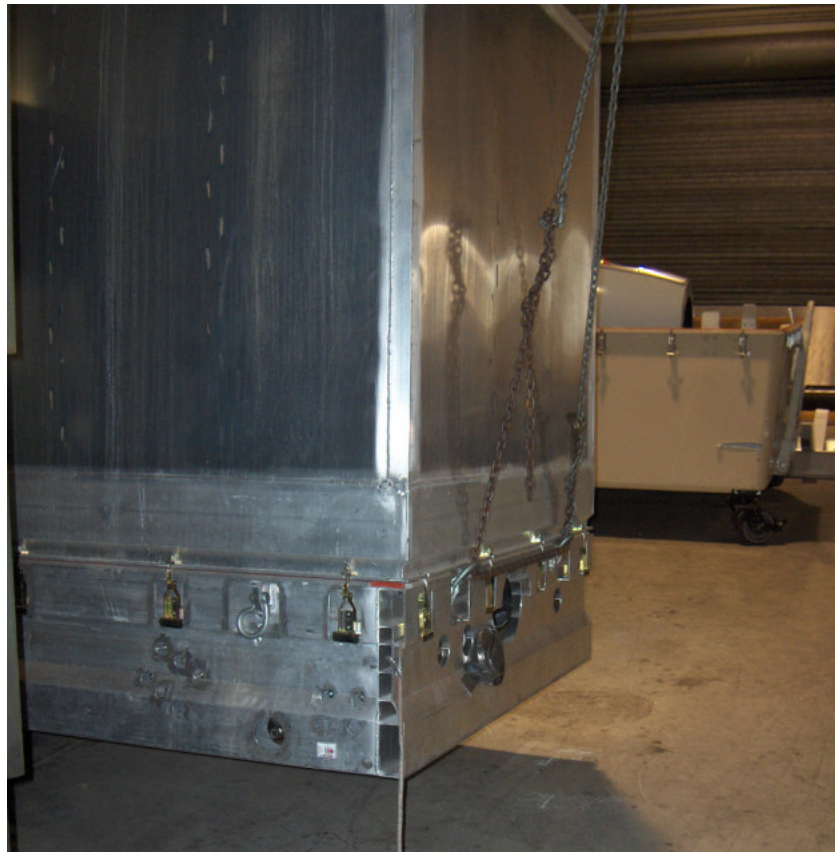
Figure 6. Rotational corner drop (view from aft end).
