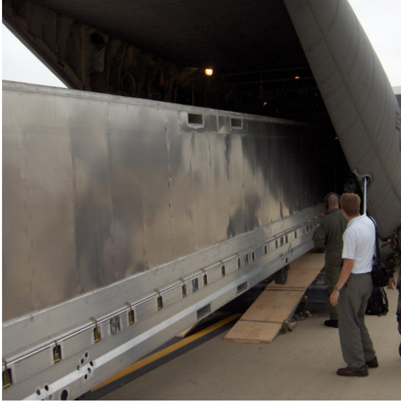
Figure 9. Container being winched up the C-130 ramp.
