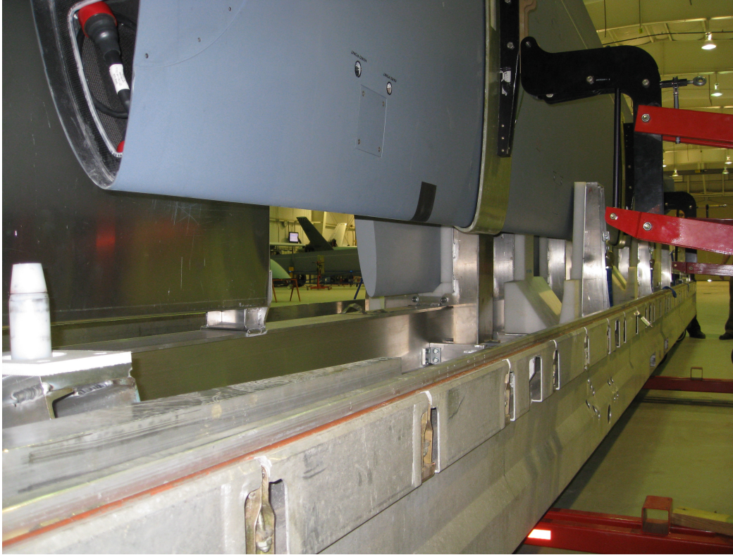
Figure 11. Wing jacks lowering a right production wing into the container base.
