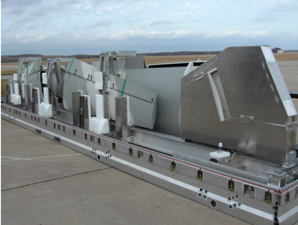
Figure 3. Container base with right test wing and diagonal tails secured (left wing and vertical tail removed)
