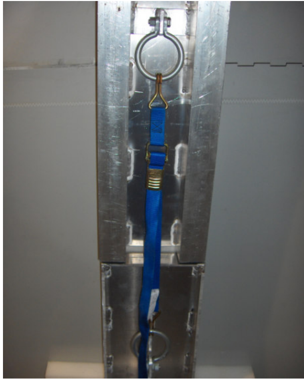
Figure 17. Cam buckle strap for L-frame tie down (1 of 6).
