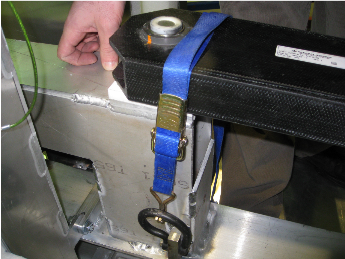
Figure 19. Diagonal tail spar tie down point (shown with production tail).
