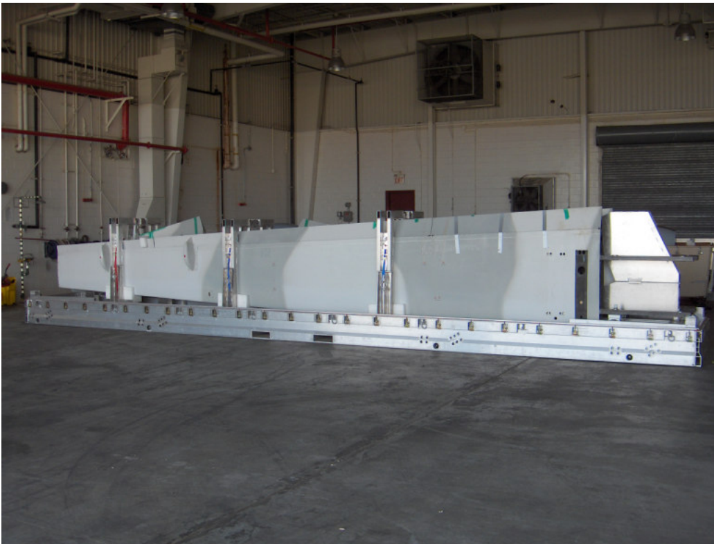
Figure 2. Container base with test wings and tails secured.
