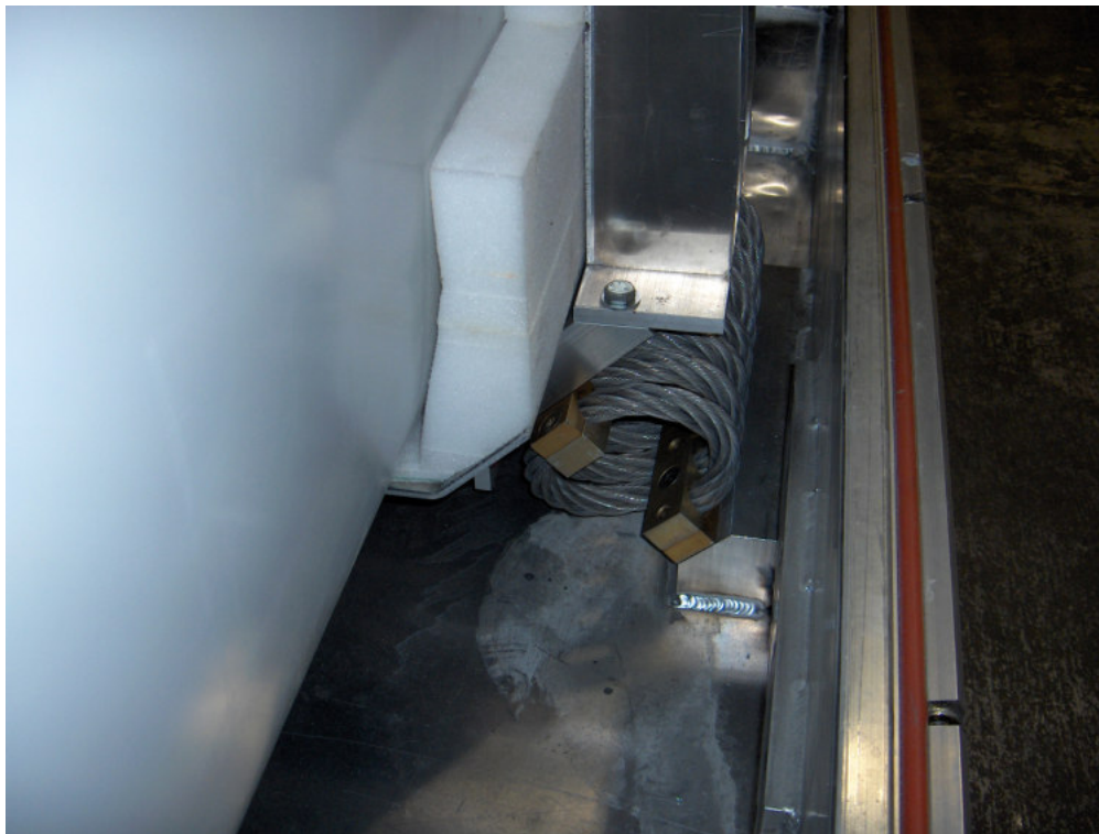
Figure 14. Lower wing cushion (white) and helical coil shock isolator.
