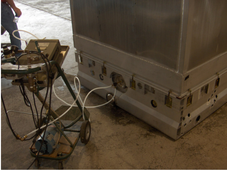
Figure 5. Pressure test set-up (for both pressure and vacuum).
