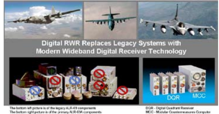
The bottom left picture is of the legacy ALR-69 components The bottom right picture is of the primary ALR-69A components
