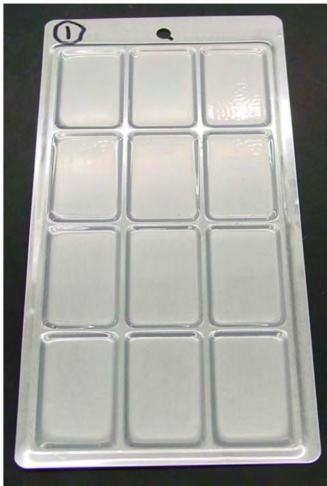
Figure 2. Photograph of the array template used to prepare coating films with a robotic film casting technique.
