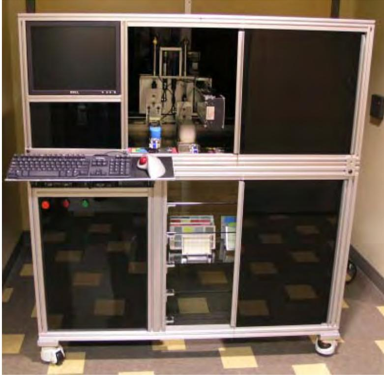
Figure 3.5-1. A photograph of the automated color and gloss measurement system built at NDSU.
