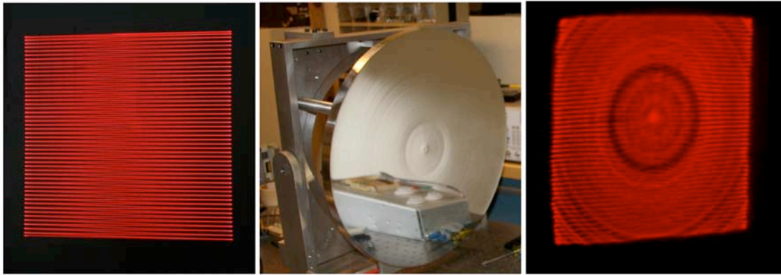
Figure 7. Test results of primary focusing mirror are shown. The left image is a Helium-Neon test scan pattern. The center image is the machined focusing mirror. The right image is the test pattern after reflecting off of the focusing mirror and projected on a white screen.
