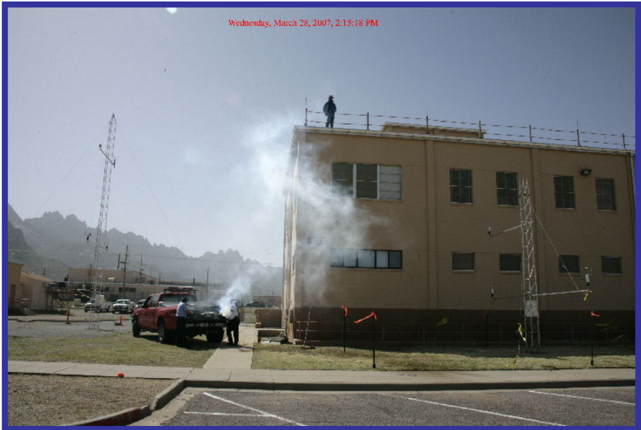
Figure 11. The W07US smoke release maps the Leeside Corner Eddy-Southeast—orange tell-tail flags on fence posts and three mounted sonics also map the Leeside Corner Eddy-Southeast; notice the tree’s absence.
