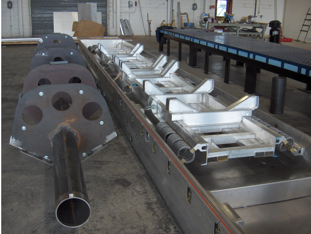
Figure 3. Mass simulator next to container cradle & base.
