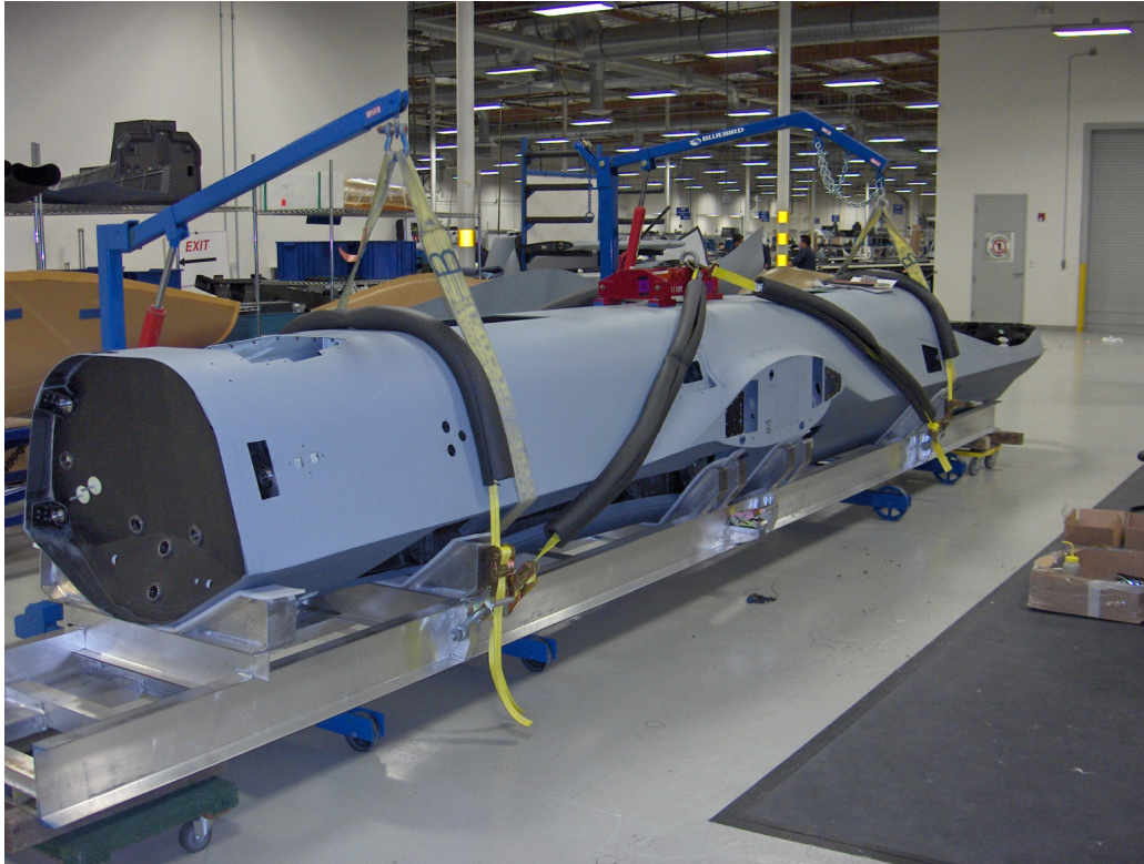
Figure 11. Fuselage/cradle fit and function testing.
