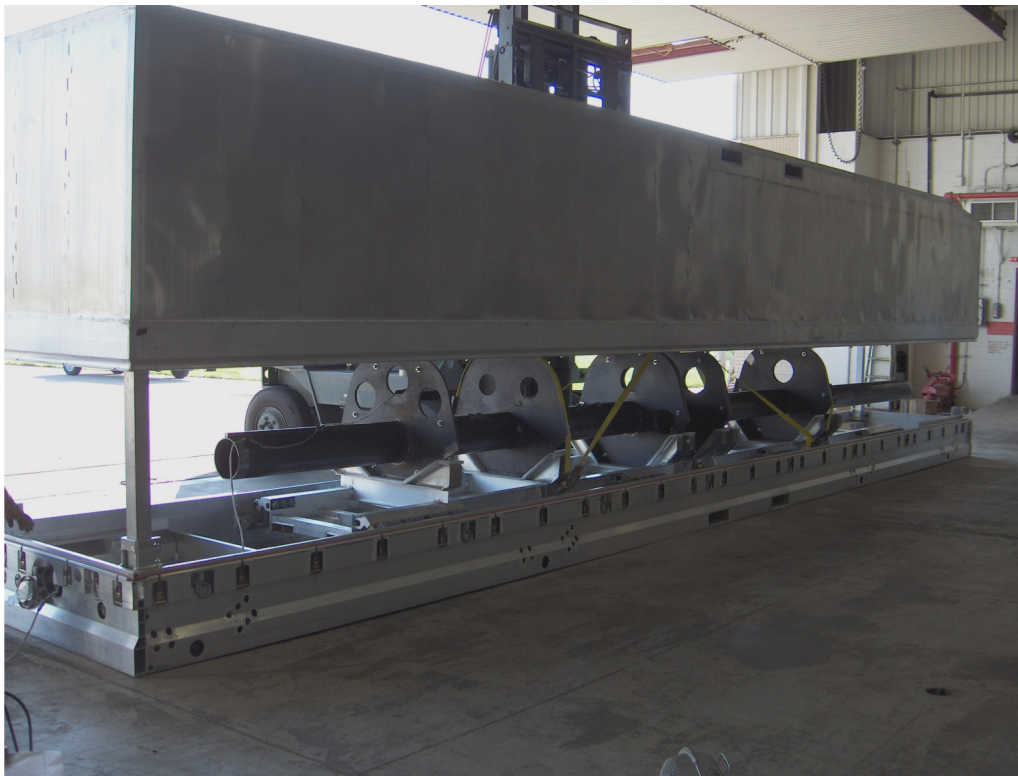
Figure 4. Mass simulator in container with cover, casters retracted.
