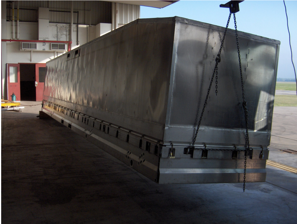
Figure 7. Rotational Corner Drop.
