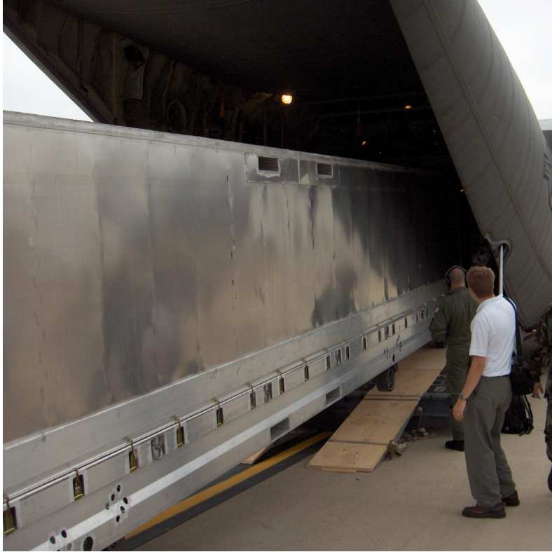
Figure 9. Container being winched up the C-130 ramp.
