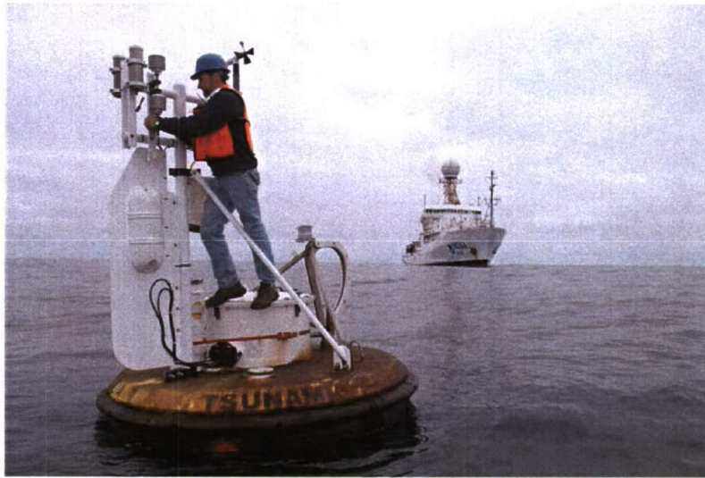
Figure 79: Service of SHOA DART buoy.
