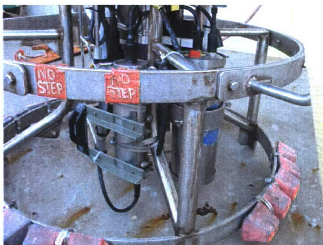
Figure 6.4: Prototype CTD strapped to frame
