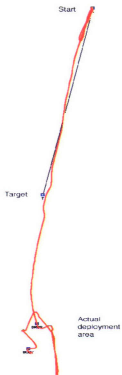
Figure 2.6: The track of RV Oceanus during the deployment of mooring F and during the subsequent survey of the anchor position. The anchor drop and buoy positions are indicated by blue squares (see next figure for details).
