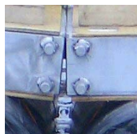
Figure 11. 1:3 Mid-scale model depiction of gap opening.
