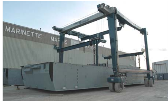
Figure 1. INLS requiring heavy-duty crane for handling.
