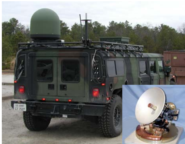
Figure 1 Example Vehicle Mounted SATCOM Dish Antenna System with Non-Ballistic Radome
