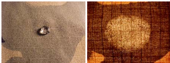
2) Moderate Water Repellent on Outer Face, Good Wicking Finish on Inner Face
