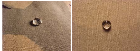
4) Good Water Repellent on Outer and Inner Faces (backlighting not necessary)
