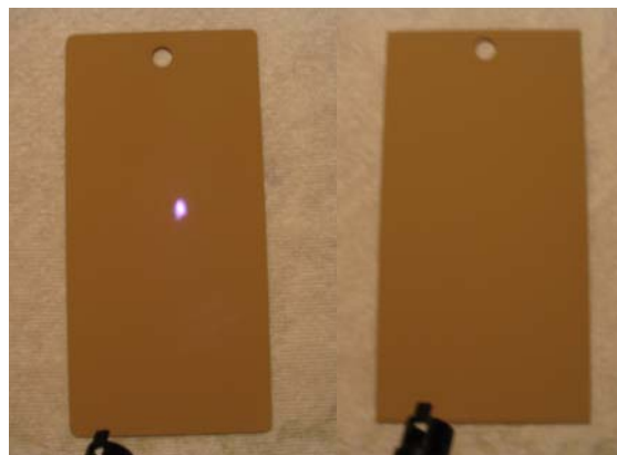
Fig. 8: Sample with phosphor is clearly visible after being excited by IR light (left), while plain CARC shows nothing (right).
