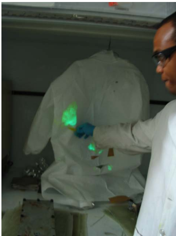
Fig. 3: Visible chemiluminescence (the green glow) showing the splatter pattern and the excellent mixing of the chemiluminescent components.
