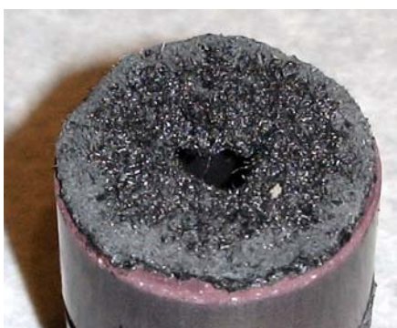
Figure 4: Igniter patch applied to pellet
