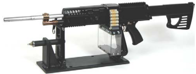
Fig. 14, CT Weapon SN1 Mounted in Test Fixture
