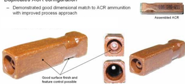
Fig. 7, Completed HITP Bodies (ACR Configuration) Fabricated Using Improved Process
