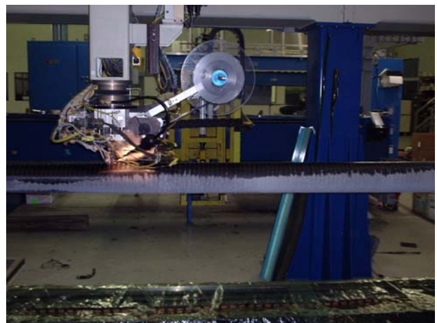
Figure 2–An axial ply being applied to the gun barrel
