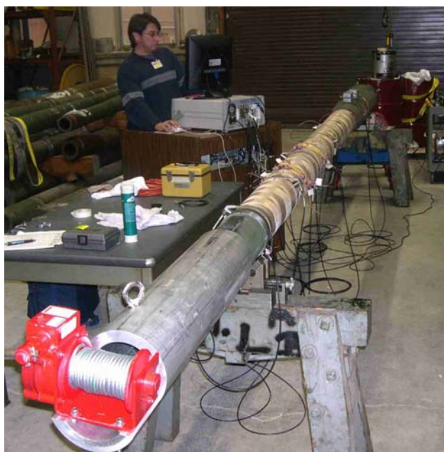
Figure 4–Acoustic Emission Test Setup
