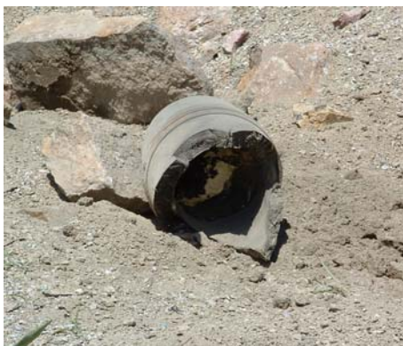
Figure 7 Large base fragment with unreacted Composition B
