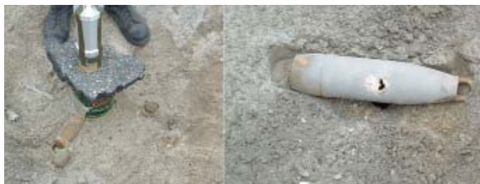
Figure 5 Initial larger design tested against an empty 105mm projectile
