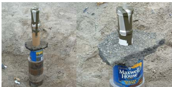
Figure 3 81mm charge at 3 CDs of standoff and 66 mm charge at 1 CD of standoff
