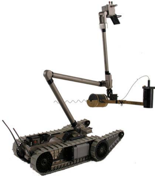
Figure 11 Robot with remote emplacement assembly
