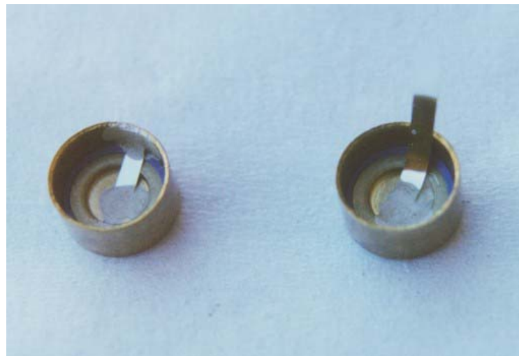
Figure 2 – Alternate (Exploding Foil) Electric Primer Configuration
