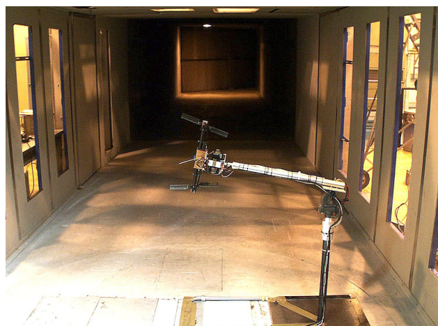
Fig. 1. Tiltrotor Descent Aerodynamics test in the Ames 7- by 10-Foot Wind Tunnel.
