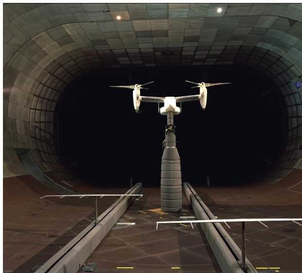
Figure 6. The FS TRAM installed in the 40- by 80-Foot Wind Tunnel showing the acoustic traverse rails and microphone wings.
