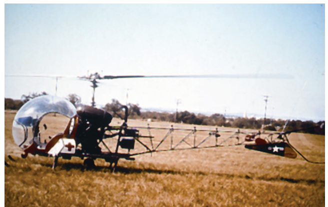
Fig. 1. The use of helicopters, as shown here, for the rapid transport of casualties from the site of injury to definitive care facilities was first begun by the U.S. Army in the Korean conflict. The patient was secured to a metal frame fastened to the outside of the helicopter. The red cross is affixed to the metal shield that protected the patient’s head during transport.
