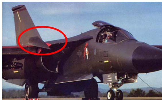
Figure 11: F-111 aircraft with vortex generator (circled) deployed to improve flow over wing gap.
