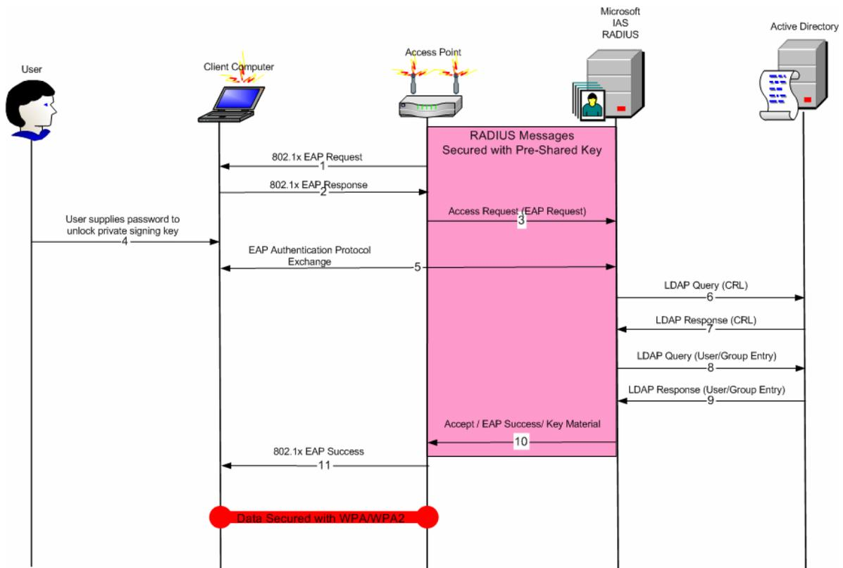
Figure 4-WLAN Authentication
