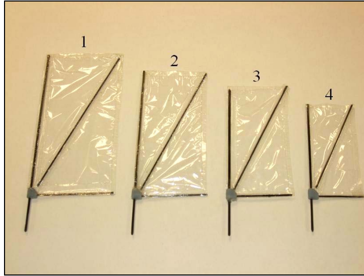
Figure 29: Flapping Wings Used For Testing
