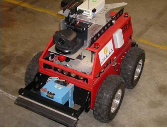
Figure 1. One of the current team members – a modified ATRVJR platform from iRobot.
