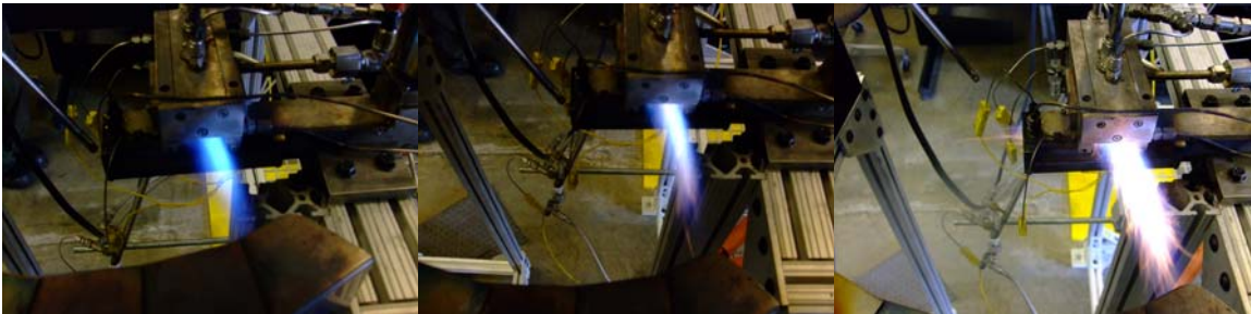
Fig. 60. UCC flames, \phi = 0.7, 1.0, and 1.6 (air ratio = 3.5, fuel = 0.0299 kg/min, airflow varied)
