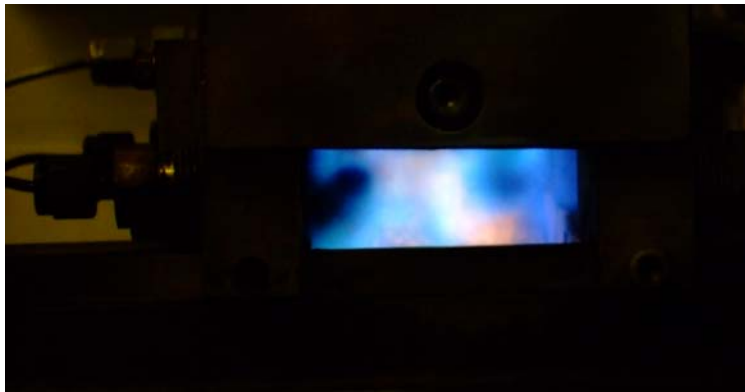
Fig. 62. Picture of flame inside UCC cavity
