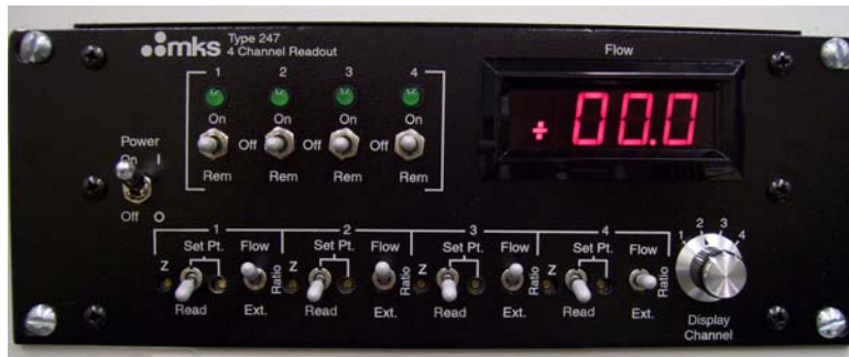
Fig. 27. MKS 247D four channel power supply/readout
