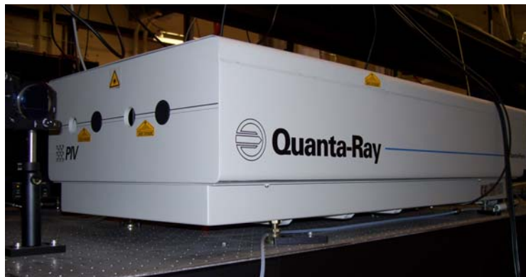
Fig. 1. Quanta-Ray PIV-Series dual pulsed Nd:YAG laser
