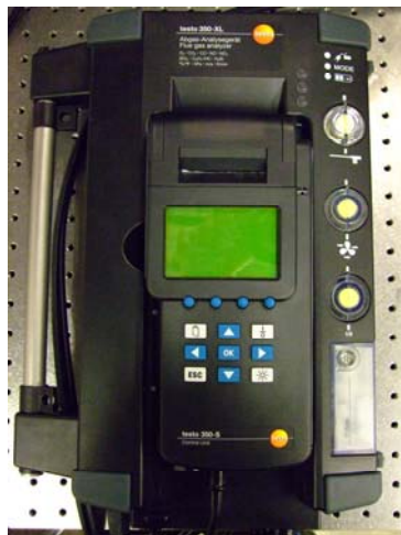
Fig. 35. Testo 350 portable emissions analyzer
