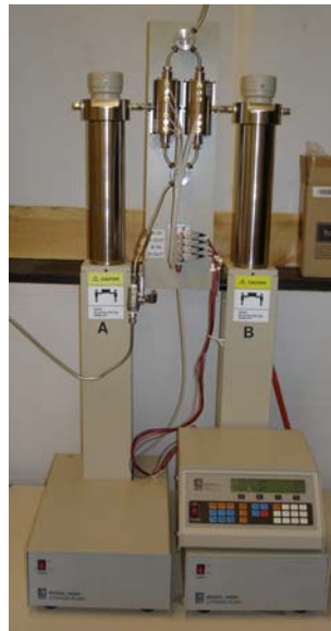
Fig. 33. ISCO dual syringe fuel pump (Ref. 3)
