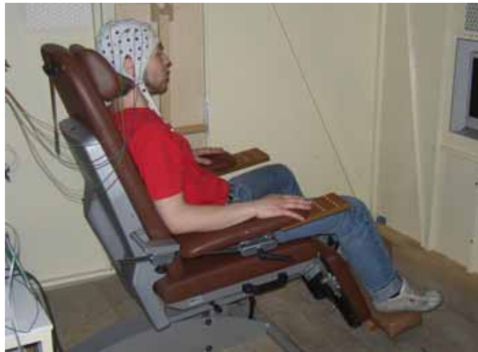
Figure B.4. Live demonstration of navigation in a virtual maze. Navigation was based upon asynchronously-detected, event-related synchronizations and desynchronizations.
