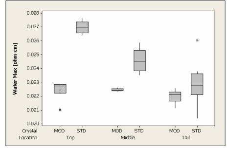
The figure displays the resistivity ranges obtained for the top, middle, and seed end (tail) thirds of two 4H n+ SiC boules. The crystals were grown under identical conditions with exception of the source. The crystal grown with the modified source (MOD) shows consistently lower resistivity and lower within crystal variation.
