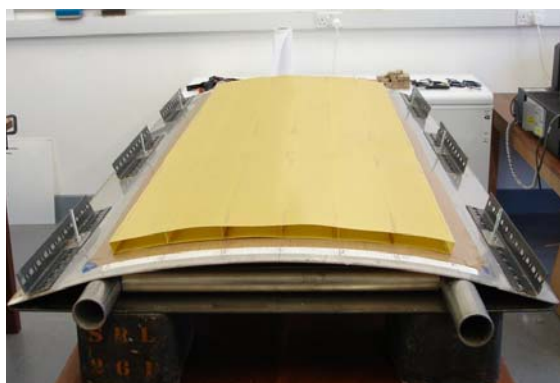
Figure 15 Mould Tool used for second structure
