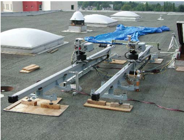
Figure 4: ADS tests at scale 1/4 on physical simulators (outdoor tests; on the left: physical simulators of the platform (left) and UAV (right), on the right: ADS and simulators command consoles)
