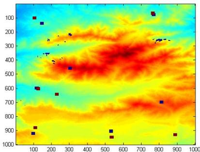
Fig. 1. The elevation data is used to define the penalty function  $f$ . The higher the area, the lower the probability of finding a sensor there. Note how the blue squares, marking the original sensor locations, move to the red squares located at lower elevation regions. The elevation map goes from dark blue, representing low elevations, to dark red, representing high elevations. The blue spots are zones of holes in the elevation information.
