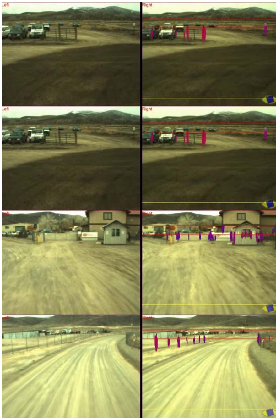
Figure 6: Images showing left and right images of different situations; on the right images, colors show the presence of detected obstacle: different colors indicate different distances. Posts—including even fence posts— and thin poles are correctly detected.
