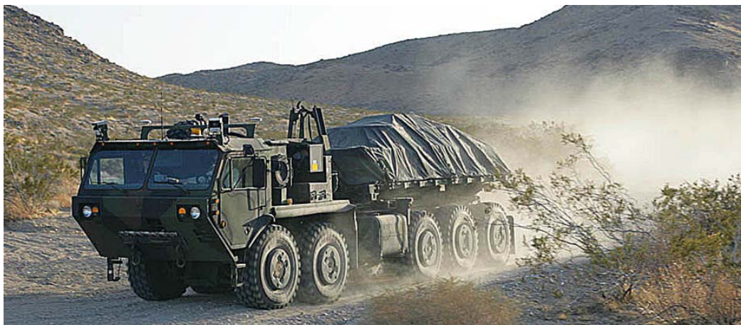
Figure 9: Autonomous PLS operating off-road with full load
