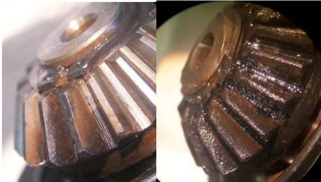
Figure 14 – Seeded Corrosion Faults (left – mild, right – severe)
