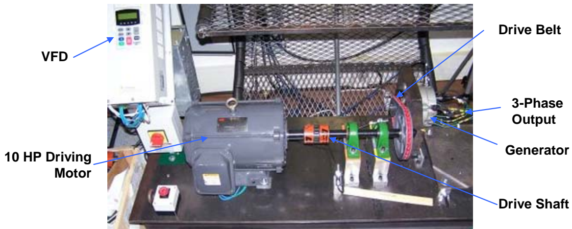
Figure 6 - Generator Test Stand Overview
