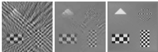
Fig. 1. Reconstructions of the phantom in Figure 2 from just 11 noiseless projections extended over 120 degrees. FBP (left), a total variation based method (center), and the results by our proposed method (right).
