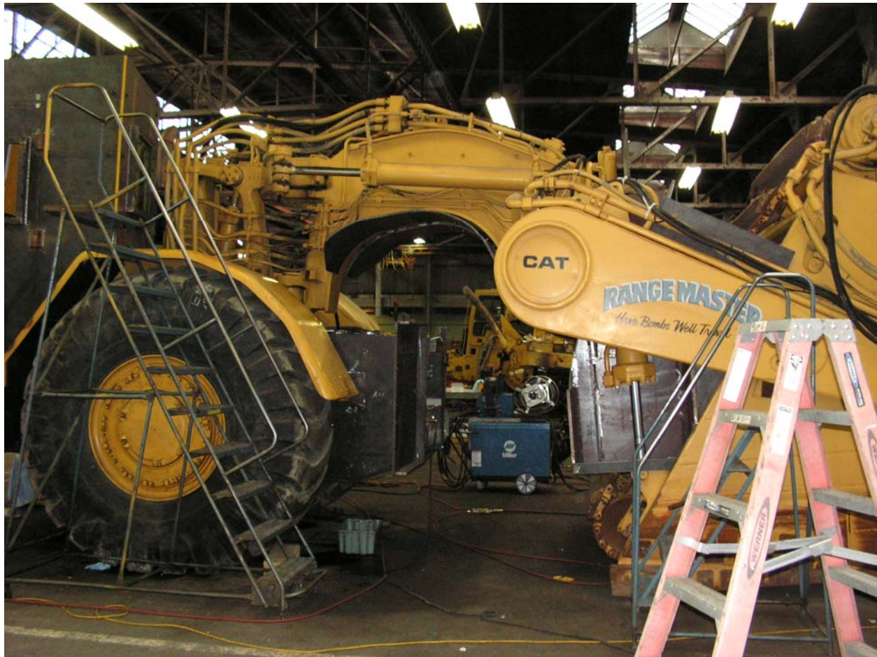
Figure 12: Phase II Armor Installation (Note Steel under Neck, behind Engine and Depth Ram)
