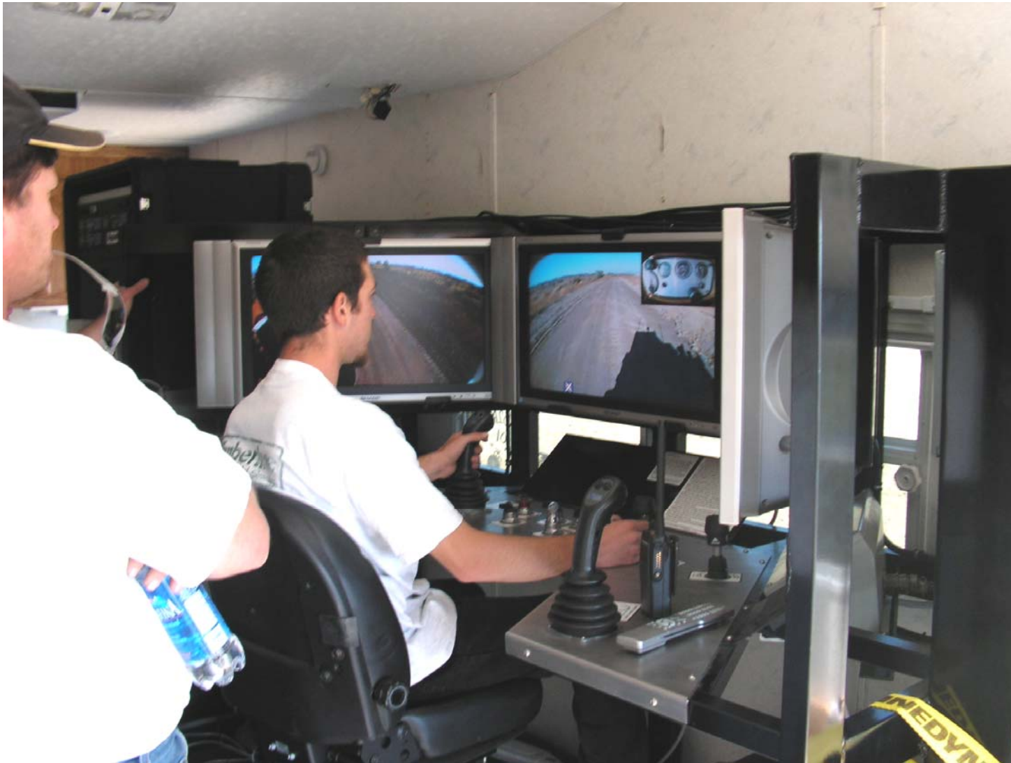
Figure 21: Remote Control Platform Video Monitors and Control Station
