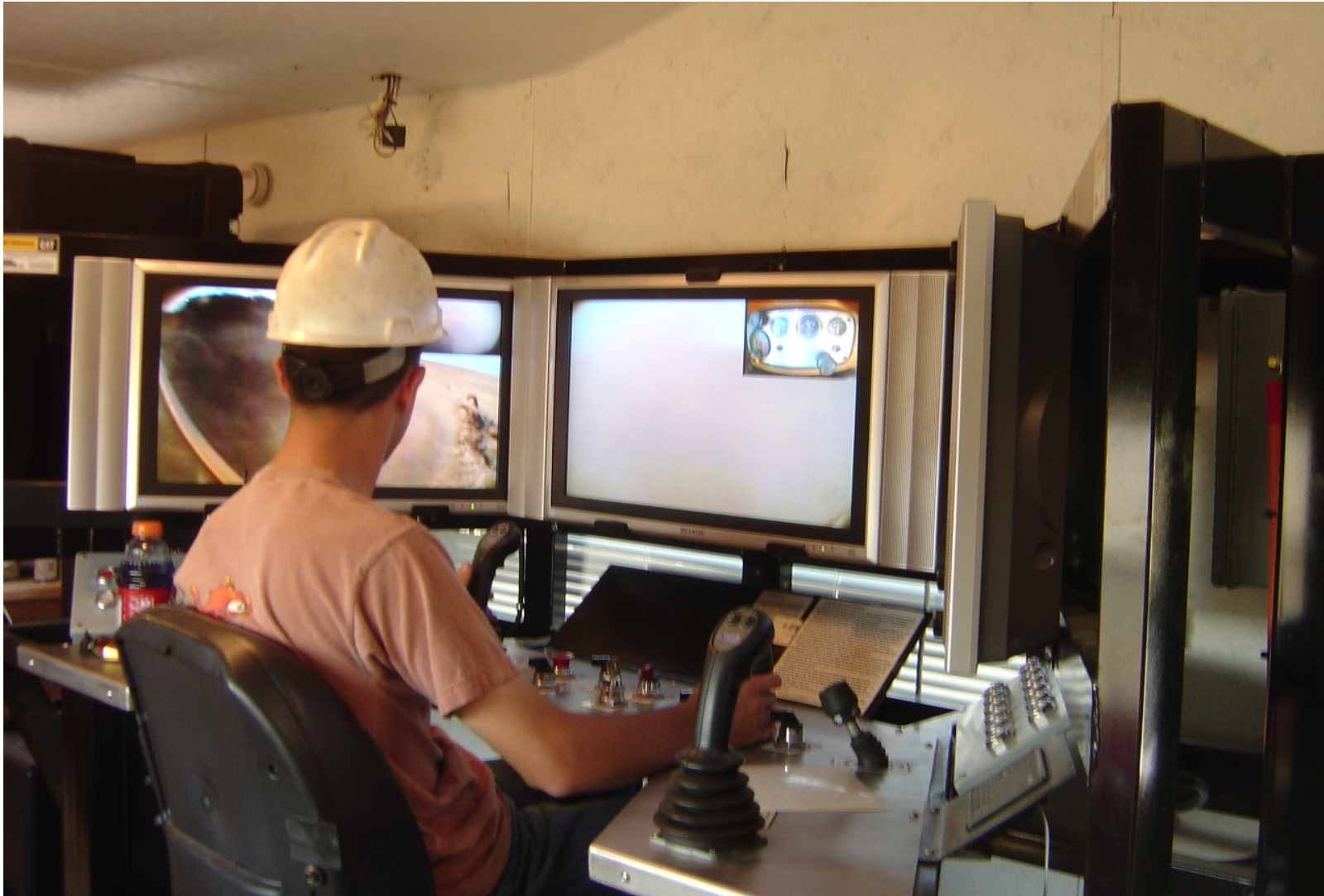
Figure 18: Video Monitors inside Remote Control Platform
