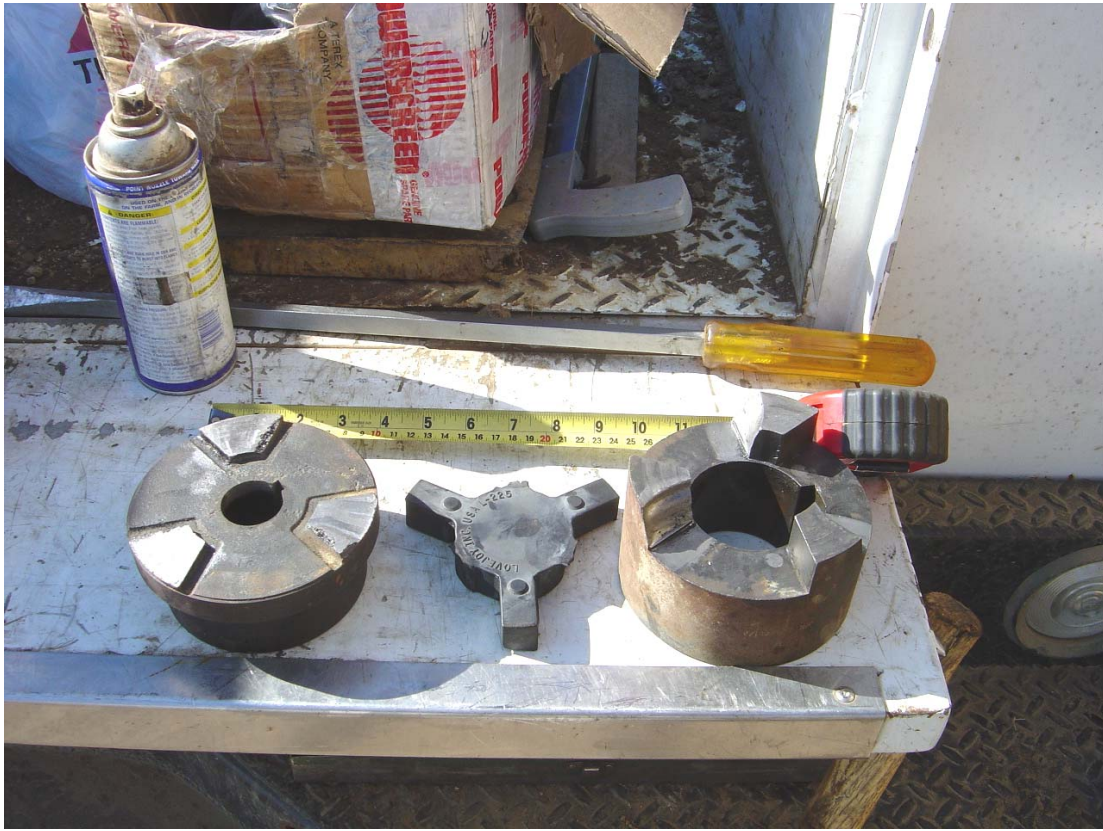
Figure 36: Broken (left) and Replacement Shaker Coupler (right)
