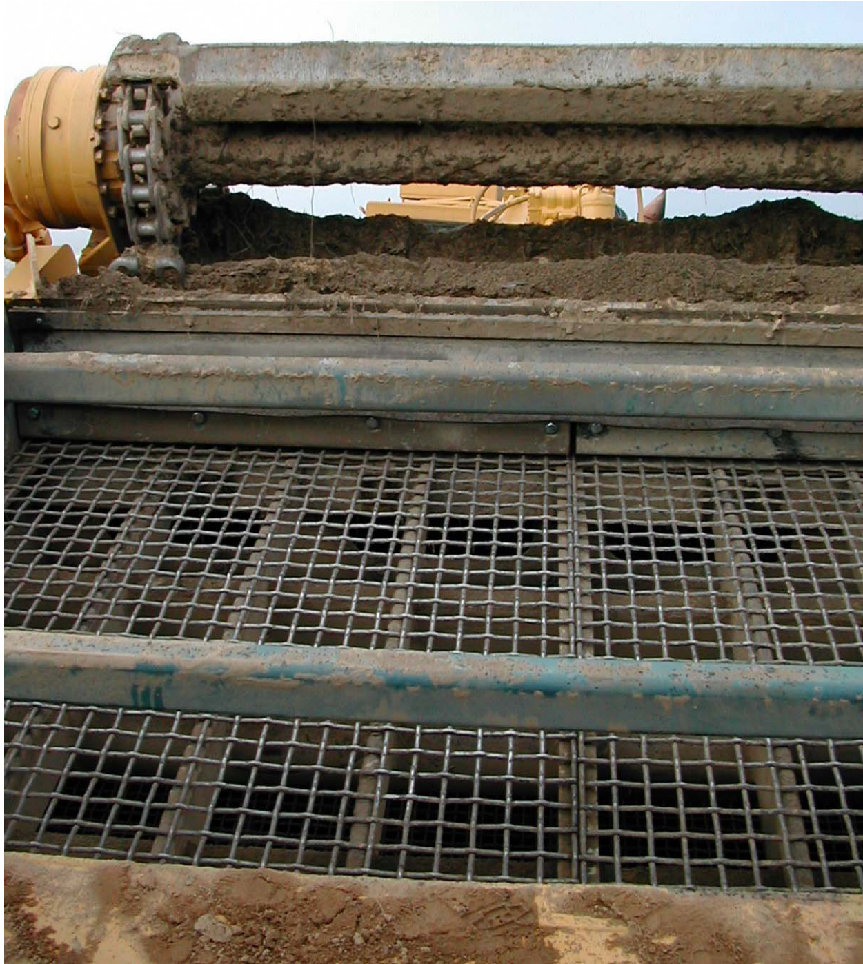
Figure 8: Screening Unit with Phase I Demonstration Fine Screen
