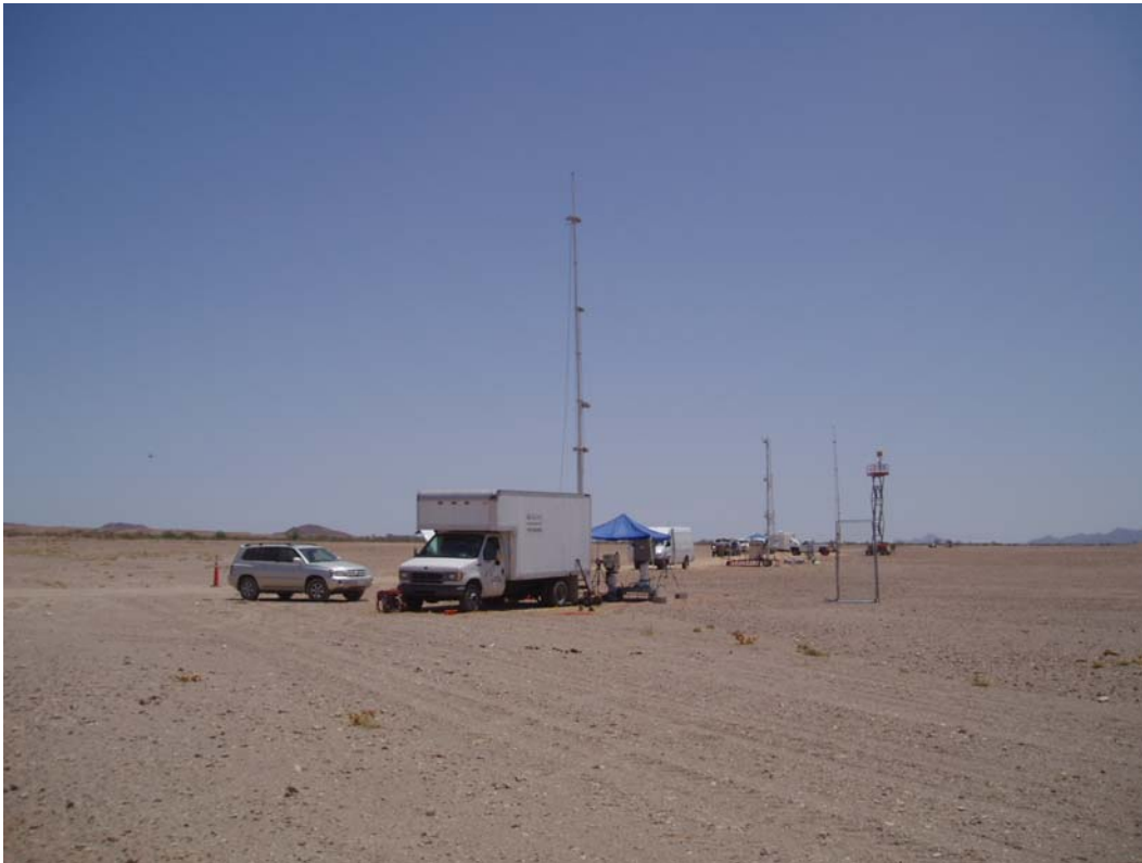
Figure 2. The instrumentation set up to measure dust emissions generated by the helicopter. The three visible towers comprise the DRI flux tower system and the optical remote sensing instruments (FTIR) are located by the panel truck. Their infrared beams are aimed at retro-reflectors on the scissor jack. The micropulse lidar is visible behind the scissor jack.
