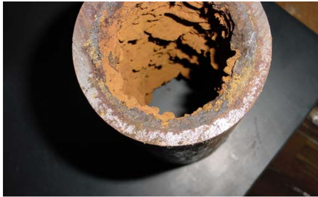
Figure 7. Iron oxide and filming amine buildup on feedwater piping.
