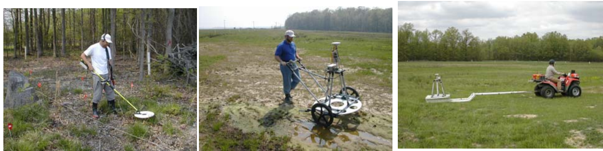
Figure 3. The GEM-3 Can Be Handheld, Cart- or Sled-Mounted, and Pushed or Towed.
