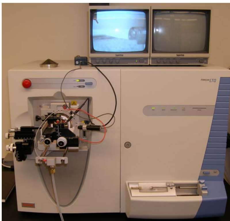
Figure 1 – Photograph of the Prosolia Omni Spray TM ionization source mounted onto the ThermoElectron LTQ MS system
