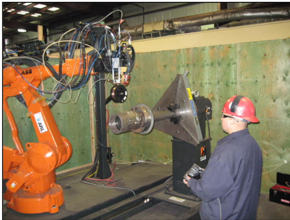
Figure 14. Photograph showing the operator jogging the robot to teach the approximate joint location.
