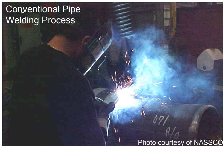
Figure 1. Photograph of the conventional pipe welding process.
