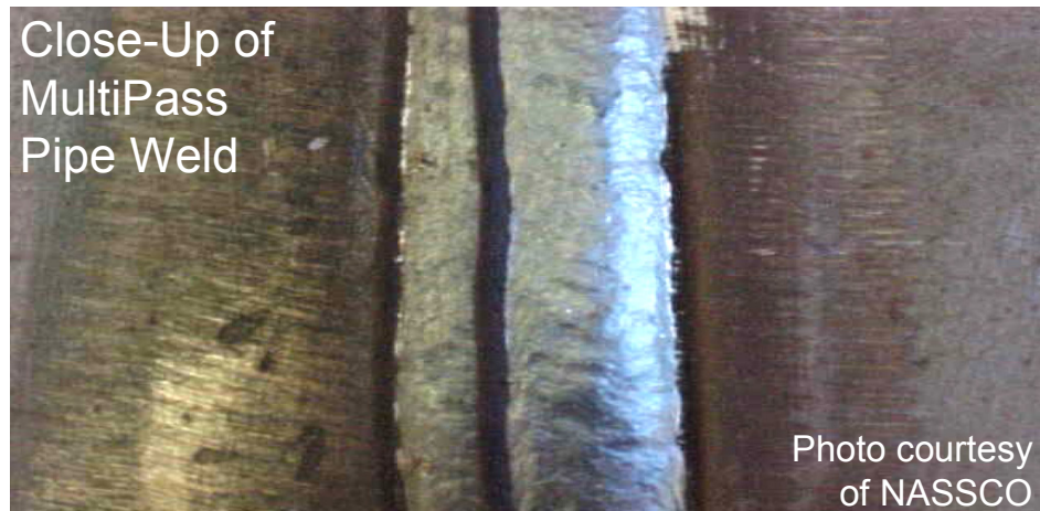
Figure 2. Close-Up photograph of multipass pipe weld.
