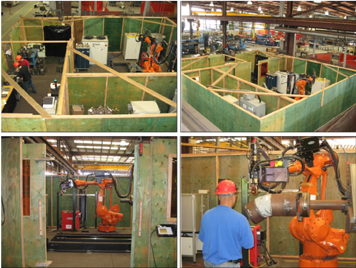
Figure 10. Photograph of the outside of the hybrid pipe welding system enclosure at NASSCO shipyard pipe shop.
