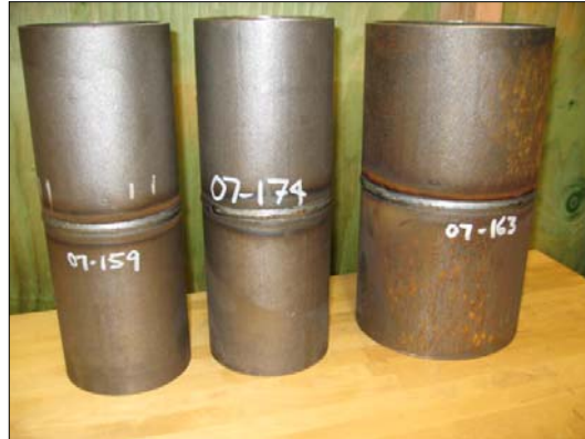
Welded test samples completed 4" sch. 40 / 4" sch. 80 / 6" sch. 40
