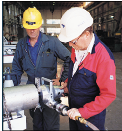
Figure 60. Example of portable pipe edge bevelling machine (source: TriTool website).
