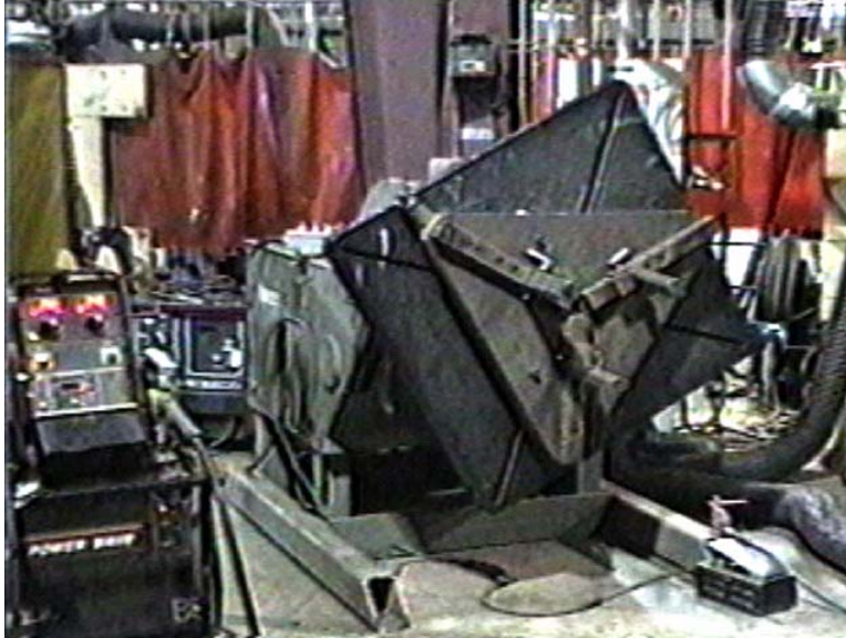
Figure 13. Image of Rotary Positioner shown as a possible example only (from NASSCO).
