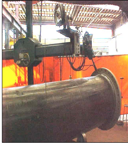
Figure 12. Image of Weld Head Manipulation System shown as a possible example only (from NASSCO).
