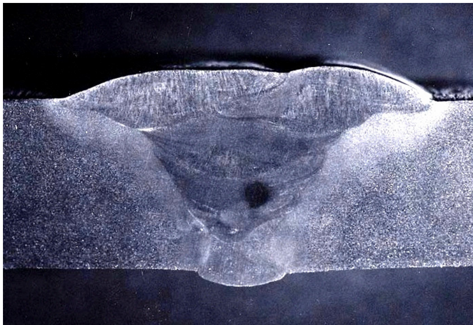
Figure 3. Cross section of conventional multipass pipe weld with 12.7 mm (0.5 in) thickness.
