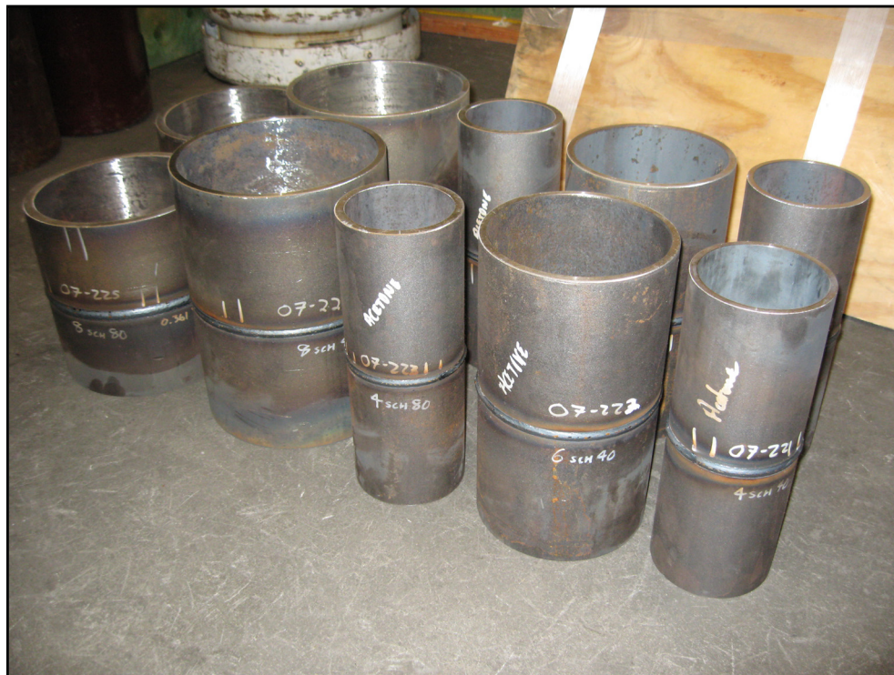
Figure 67. Photograph of pipes joined with a hybrid laser-GMA weld for the small production test run time study.
