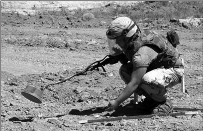
PFC M. Smith marks mines and unexploded ordnance at Bagram Air Field.
