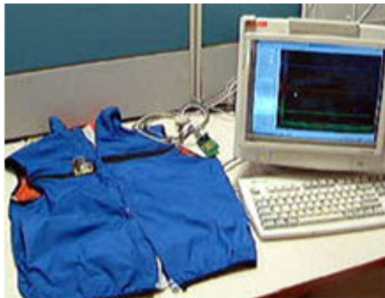
The jacket is fitted with a sensor and a Bluetooth transmitter that communicates with a receiver.
