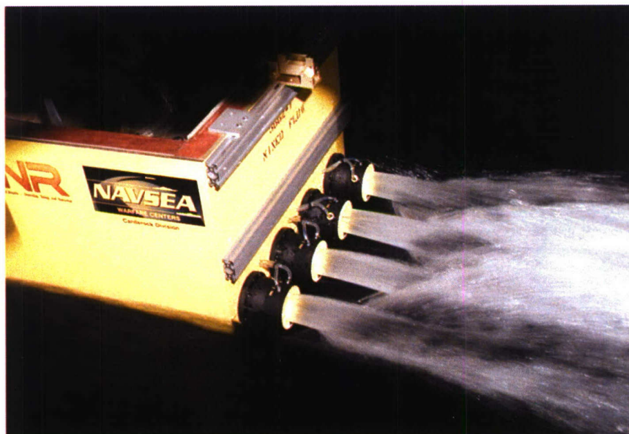
Mixed-Flow waterjet Model 5662-1 powering run at 36 knots ship speed
