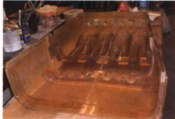
Fig 2. Model 5662 waterjet stern plug assembly
