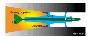
**Figure 2:** Pressure builds behind the sabot and propels the projectile down the gun tube.<sup>54</sup>
