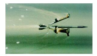
Figure 3: A representation of the final stage of sabot separation from the penetrator.<sup>59</sup>
