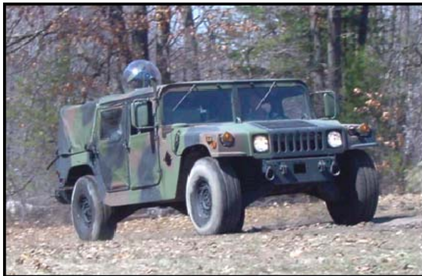
Figure 2. HMMWV test vehicle with small, parabolic COTM antenna [5].
