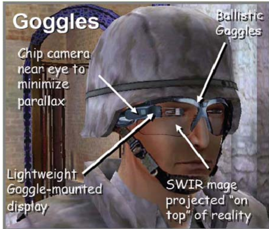
Figure 9. SWIR cameras are being integrated into current field goggles to image laser designator and rangefinder spots (From [17])
