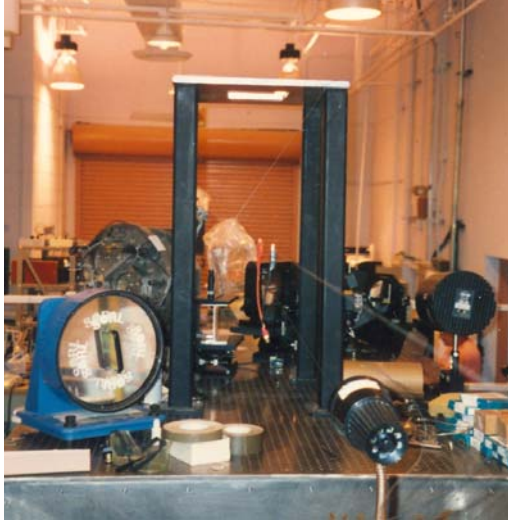
(a) (b) Fig. 43. Details of Wire-Guided Flight Set-Up Showing the Anchored Wire Attaching to the Standoff on the Optical Bench (a) and Looking Back From the Tower to the Open Window (b)
