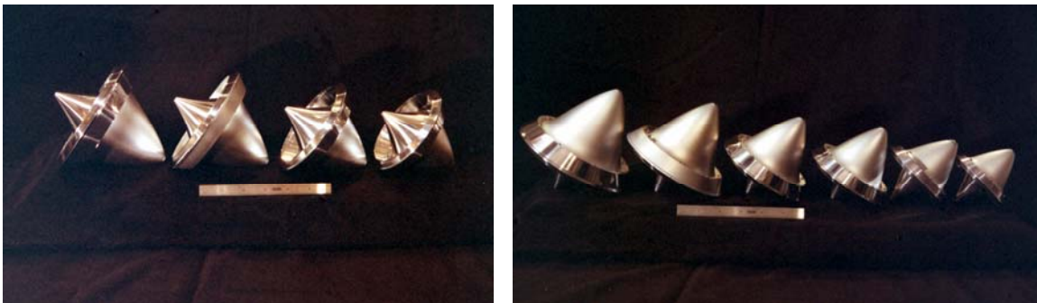
Fig. 66. Two Views of the Scaled Family of #200 6061 T6 Aluminum Lightcraft (21)
