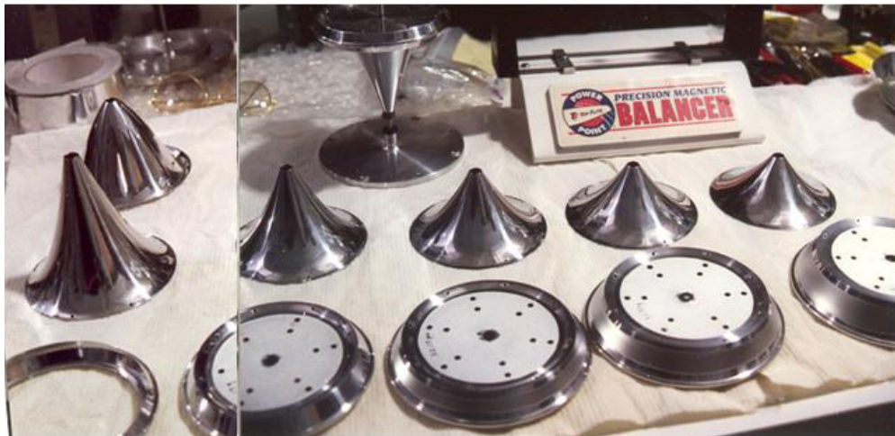
Fig. 54. Composite Picture Showing Paraboloids #100 to #300 with Titanium Shroud on Far Left
