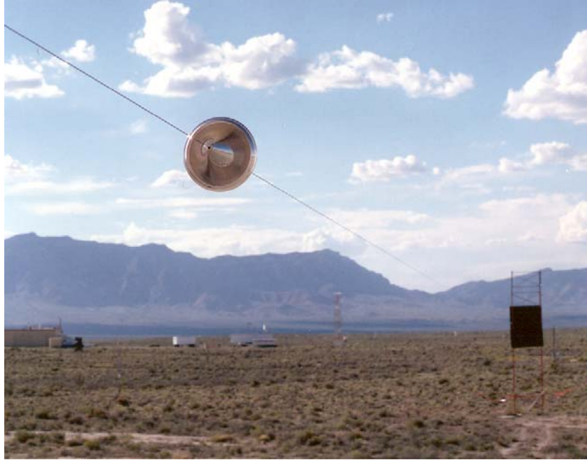
Fig. 58. Lightcraft Mounted on 400 ft Horizontal Wire Tied to Beam Stop
