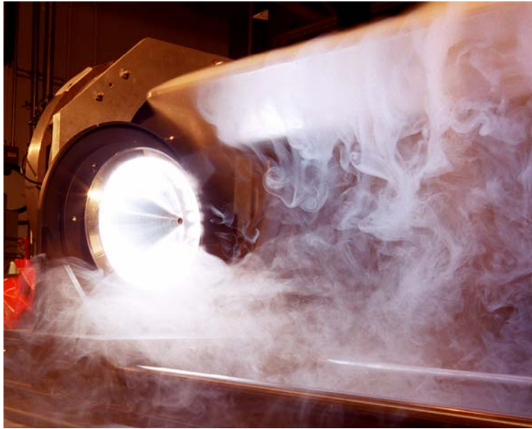
Fig. 73. Exhaust Field Visualization Test Using Vapor Created by Pouring Liquid Nitrogen Into a Bath of Water (The Water Bath is Above and to the Right)
