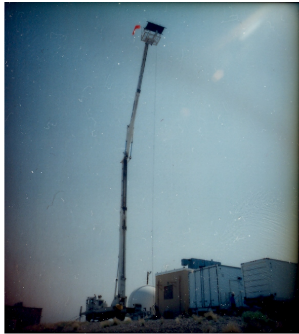
Fig. 79. Condor Crane with Wind Sock and Wiffle Ball Measurement Line Attached
