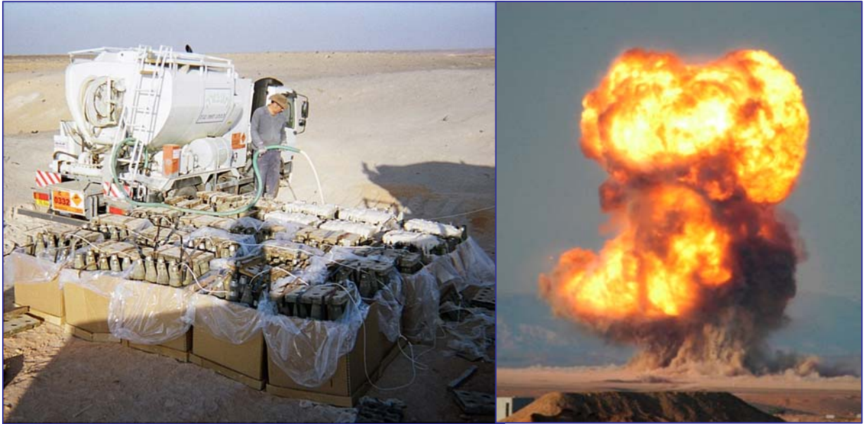
Figure 22. Sayarim ammunition explosion on Dec. 6, 2005 (Ex.17). Industrial explosive (ANFO-like emulsion Henamit) was added to provide full demolition of the shells (left). The right photo is made from the distance ~3 km, with a large zoom (courtesy of Y. Hamashdyan of IDF).
