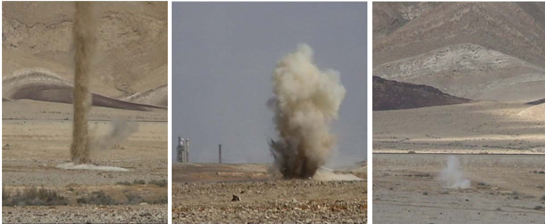
Figure 56. Surface effects during detonation for Ex.1 (a), Ex.2 (b) and Ex.3 (c).
