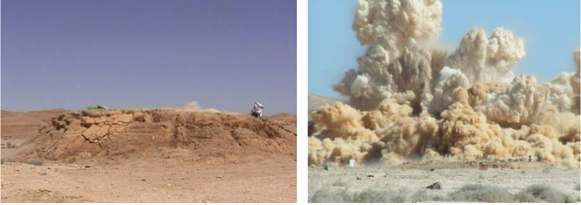
Figure 13. Sayarim buried explosions: (a) ground uplift for the 2-ton shot (video snapshot ~1 sec after detonation); (b) view of the largest explosion 32.5 tons.
