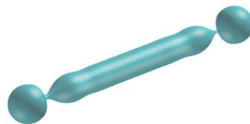
Figure 20. Bubble behavior in a vortex flow field: core radius = 4.51 mm, circulation = 0.2123 \text{m}^2/\text{s} ; \sigma = 1.72 ; U_\infty = 10 \text{ m/s} ; initial radius of the bubble = 750 \mu\text{m} . Three-dimensional view of the bubble just before splitting predicted by 2DYNAFS ® .
